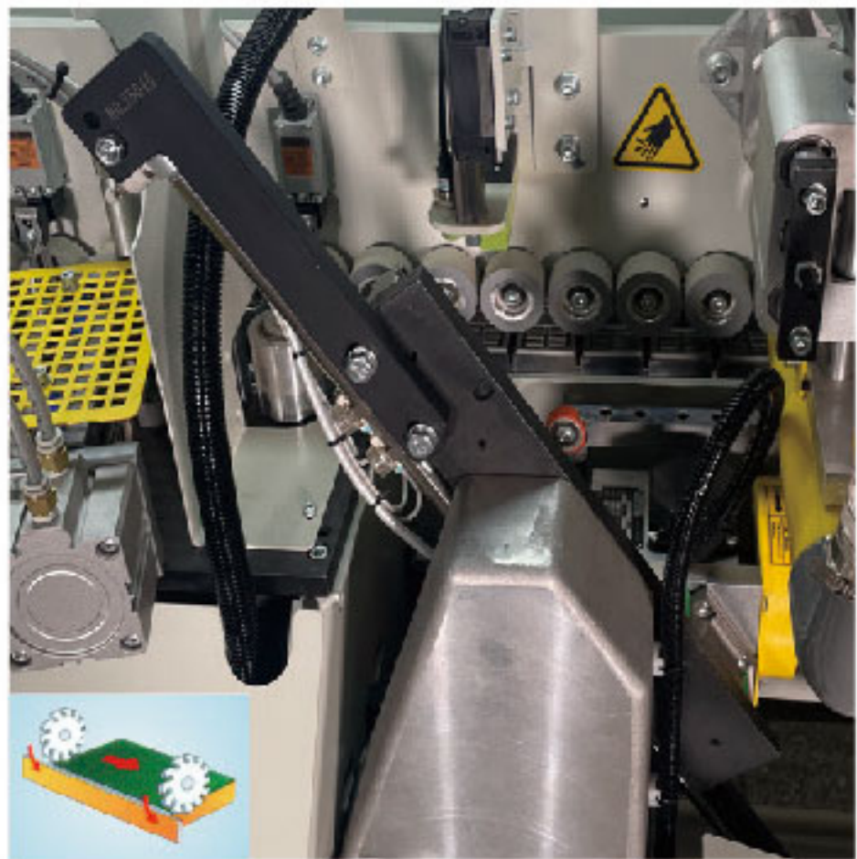
End Cutting The end cutting with 2 independent saws, with one high frequency motor running at 12000rpm.Linear guidance ensures the highest level of precision.
