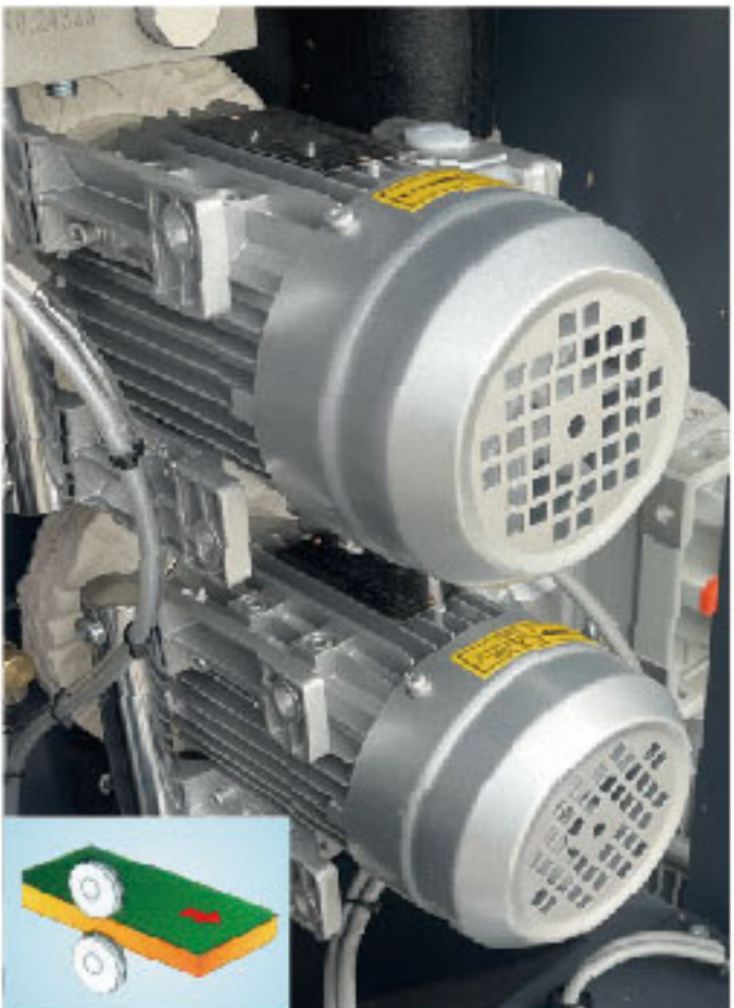
Buffing Unit Effecttively clean off glue residue on the edge
