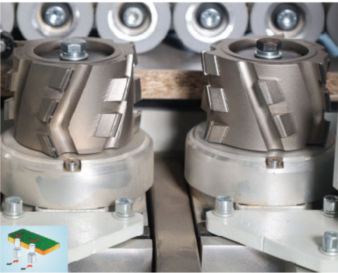
Pre-milling Unit Two high speed knives can make sure the workpiece keep the same size.
