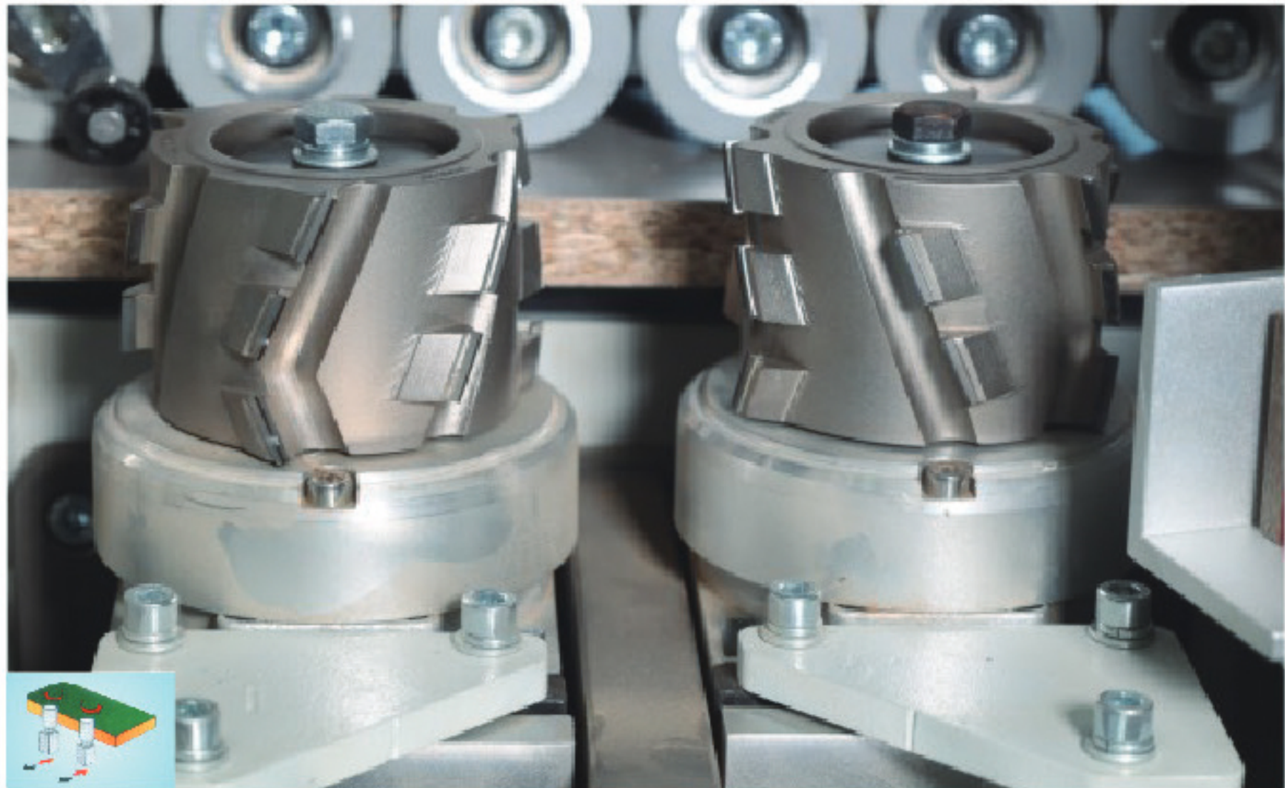
Pre-milling Unit Two high speed knives can make sure the workpiece keep the same size
